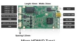
Micro HDMI(D Type) **Encoding Board Interface**
