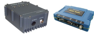
FGR2-15瓦 (15.1x11.5x6.2/17.1x11.2x3.2cm, 900/680g) (153.6k/1.2Mbps, 15瓦, 232/485/422, 10.5-16V/4A, TNC)
